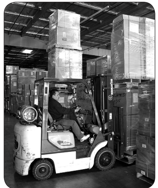
This forklift is fueled by propane.
